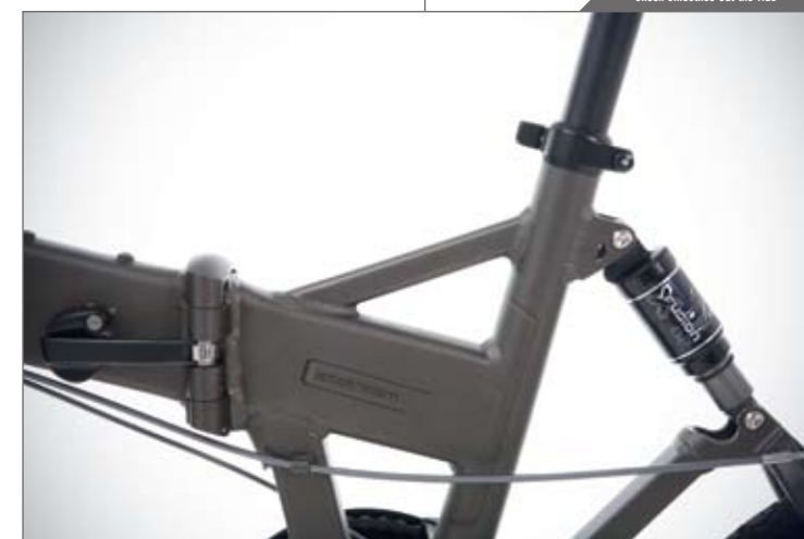
Dahon hinges are excellent and rear shock smoothes out the ride
