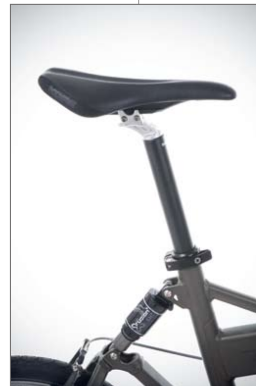
Superlight parts but 'i-beam' saddle restricts the ability to personalize
