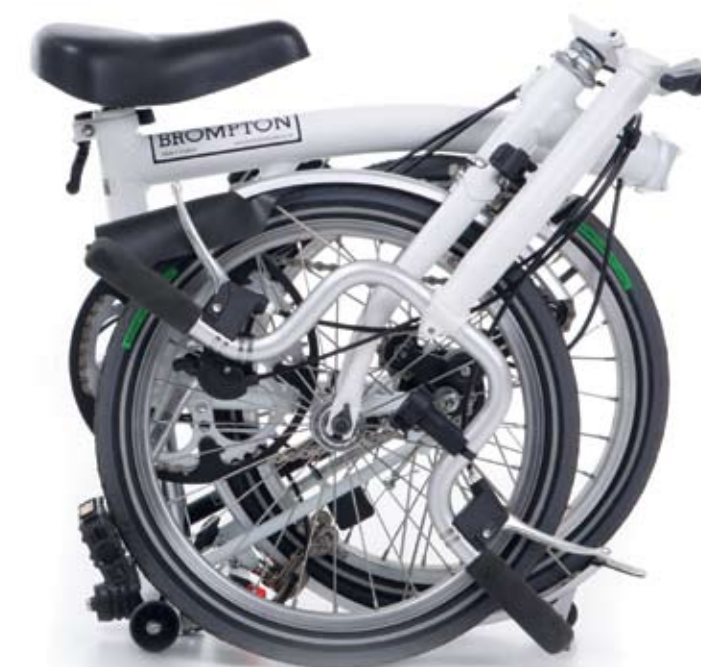
Hub gear system requires chain tension device
