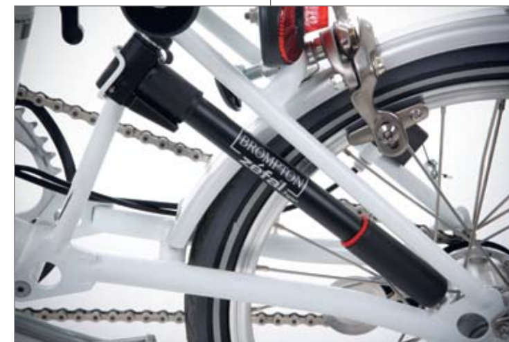
Decent quality pump already fitted to the Brompton
