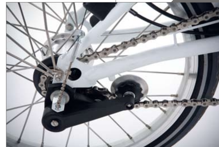
Hub gear system requires chain tension device
