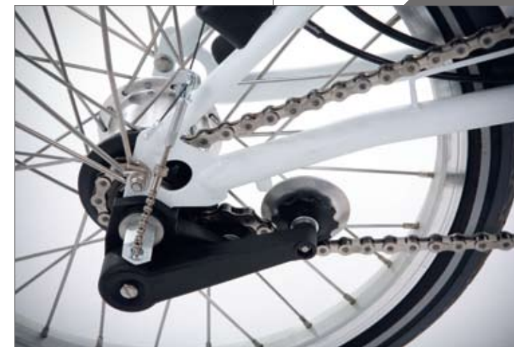
Hub gear system requires chain tension device
