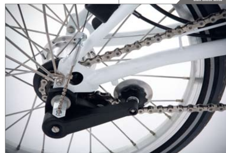
Hub gear system requires chain tension device
