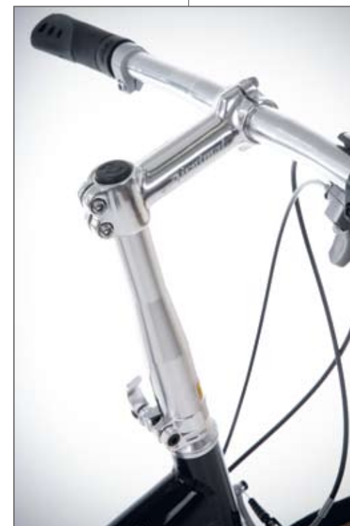
Plenty of adjustability on the Joey; most folding bike bars are fixed
