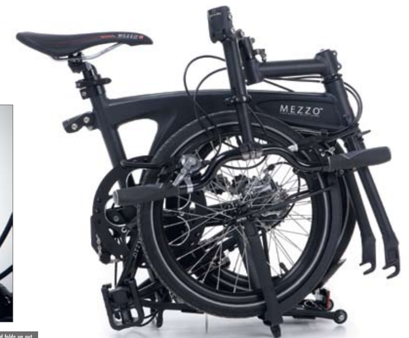
Integrated mudguard folds up out of the way with the wheel
