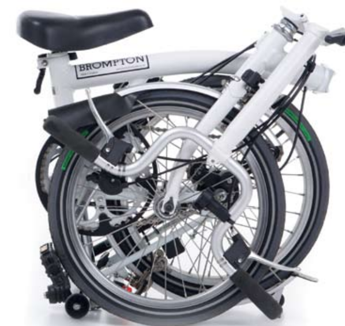
Hub gear system requires chain tension device
