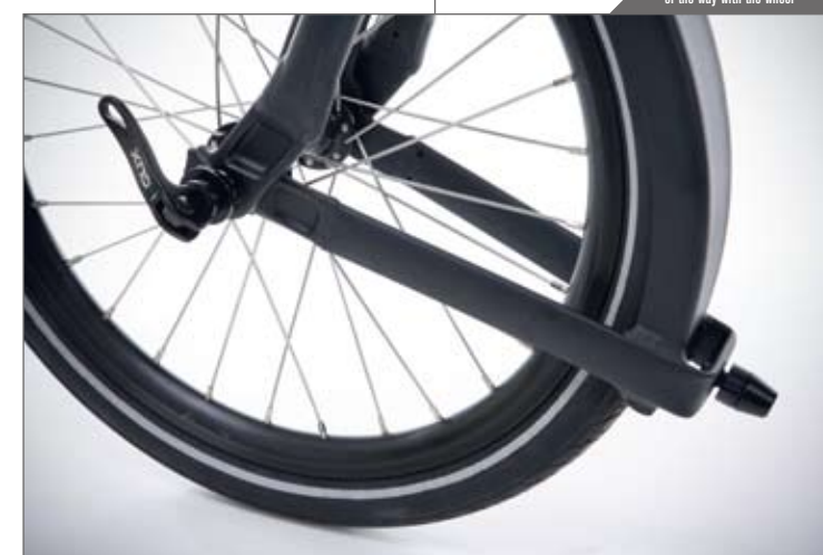
Integrated mudguard folds up out of the way with the wheel
