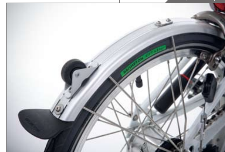
Mudguard with trolley wheel hiding the puncture resistant tyres
