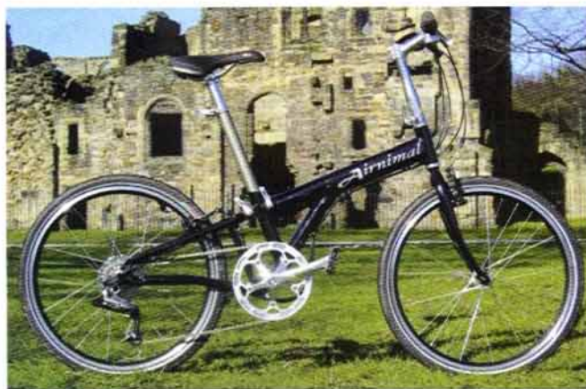
New ETRTO/ISO 507 wheelset means greater choice of tyres is available. Below right: Quick release removable bars are great for folding or even stowing the bike. Bottom right: SRAM dual-drive 3x8 hub gear and cassette means great gear range
